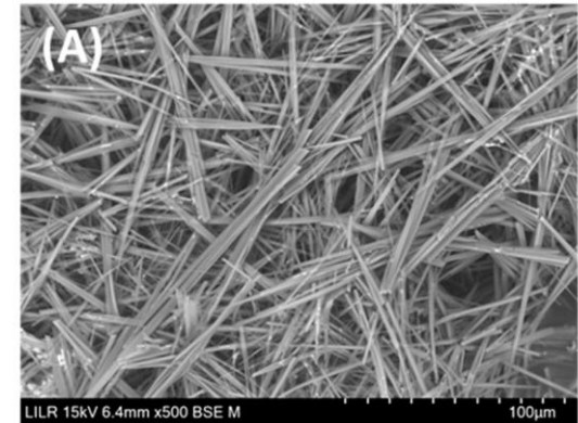
SCANNING ELECTRON MICROSCOPY OF CRYSTALS FORMED BY THE SELF-ASSEMBLY OF A METABOLITE
